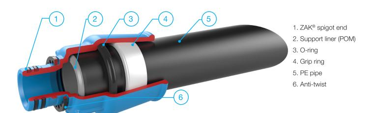
Note: For push-fit fittings in the domestic connection sector (d 25 to d 63 mm) the support liners (POM) are included at the factory. The number of support liners included is based on the number of connections.
