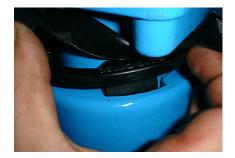
To secure the swivel socket, the supplied anti-twist device DN80 is installed in the gap between the body and the socket. If required, enlarge the gap by lifting the socket. There are notches in the body and in the socket. The anti-twist device is now inserted into these notches. Caution: Do not damage the coating!
