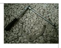
If a hydrant DN 80 with spigot end is installed in the socket, the socket must be turned to a 45° position. The hydrant is then inserted. To lock the socket, place the turning tool on the lateral bolts and turn the socket counter clockwise with the ratchet until the hydrant is locked. The anti-rotation device and dirt cap supplied must be fitted to prevent unintentional twisting and contamination.
