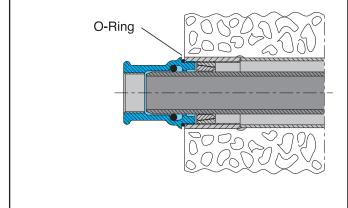
Assemble the fitting without sealant! (The o-ring between the steel pipe and fitting saves on packing)
