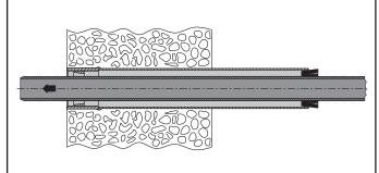
1. After fixing protective conduit in masonry walls. Pull the medium pipe in, then cut straight and chamfer.
