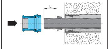
2. Slide the grip ring on while observing the insertion length (L) of the pipe end.
