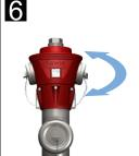
If required, turn the hydrant head to the desired position.
