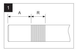
For pipes with a very smooth surface (e.g. PE-X pipes) we recommend roughening the pipe end only in the clamp area (see table) perpendicular to the pipe axis!
