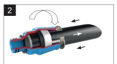
Insert extractors (Ord. No. 601-00) completely. Pull out pipe by turning it.
