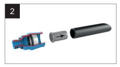
Use pipe end without notches and grooves on the surface. Cut pipe straight with sharp PE shears.
