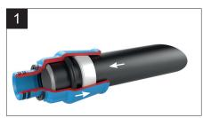
Release the load on the fitting or pipe in the mounting direction: (short jerk)!
