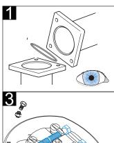
Visual inspection for damage or dirt on or in the hydrant. Dispose of opened or broken break away bolts.
