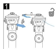
Detach cap for B- or A-coupling. Then open and flush the hydrant
