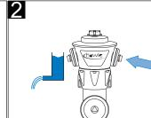
Close hydrant after use. Disconnect the A- or B- hose. Check drainage function. If the hydrant does not drain after a waiting period of two to three minutes, the blocked draining bore must be flushed free, e.g. with a hand pump.
