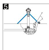
Fill up the excavation pit and compact the soil. Support the hydrant below the break away area sufficiently against the soil.
