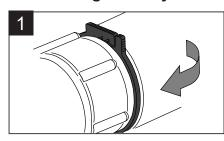
Open the interlocking of the fixing ring. Expand the fixing ring and pull it back.
