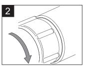
Apply approved lubricant Turn the ZAK® connection Pull back ZAK® connection to the O-rings of the spigot fitting 90° clockwise as far fitting approx. 4 mm as far
