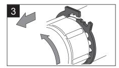
Turn the ZAK® connection fitting 90° counter-clockwise as far as it will go and pull it out of the ZAK® connection sleeve. After dismantling, check Orings and replace if necessary.
