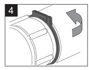
Slide the fixing ring into the gap and engage the interlocking by pressing it together. (The fixing ring can be pulled on so far that it can also be inserted later)
