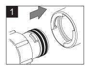
end and slide the ZAK® spi- as it will go. got end into the ZAK® socket as far as it will go.
