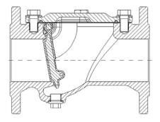
Medium: Operatin temperature: Max. Betriebsdruck: Material: Potable water / Sewage water 0° to 40° 16 bar Body and cover: GJS-400/500, Hawle epoxy powder coated Drain plug: Stainless steel Valve disc: Steel/EPDM
