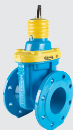
400-00G Flanged gate valve "E3", Face-to-face length, basic series 14 according to DIN EN 558-1
