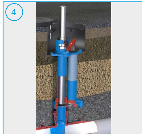
4 Install the probe through the gasket below until just before the shut-off blade.
