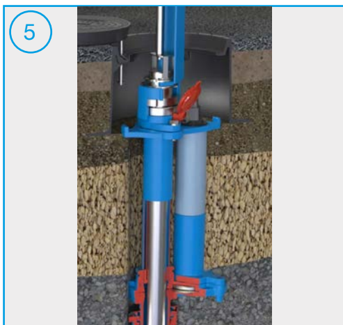
5 Put on the inserting tool, then open the underground hydrant under full operating pressure and move the sensor to its final position in the flow.
