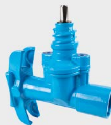
Valve saddle: Lateral drilling, shut-off effected by means of resilient-seated wedge
