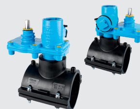
239-02G Hawlinger with upper horizontal ZAK® socket 90° to pipe direction for gas
