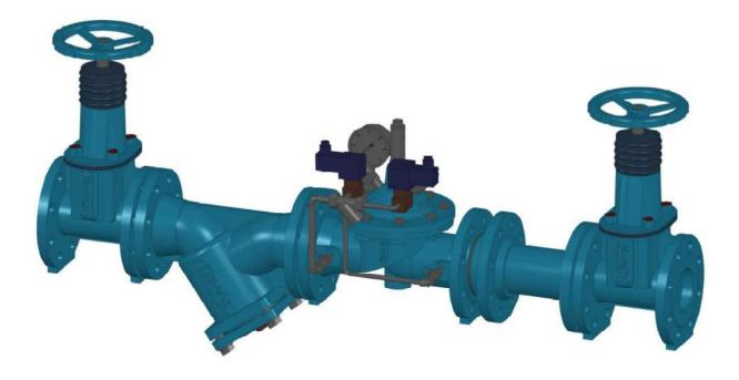
The HAWIDO must be installed horizontally with the valve cover upwards (other models available on request). We recommend that a gate valve and a dirt trap be fitted in front of the valve, as well as the mounting of a gate valve at the outlet. Before the installation, check that no coarse foreign objects can penetrate into the HAWIDO.
