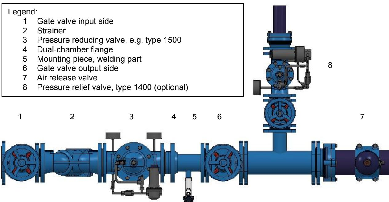
Regulating valves are normally fitted with the valve cover upwards and it is recommended that shut-off valves be fitted on both sides plus a dirt trap on the inlet side. Depending on the installation situation, a mounting adapter may also be required.
