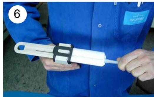
Apply the mixing tube and fix it by performing 1/4 turn.
