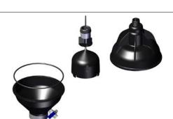
4. Lift the body halves containing the valve mechanism off each other.
