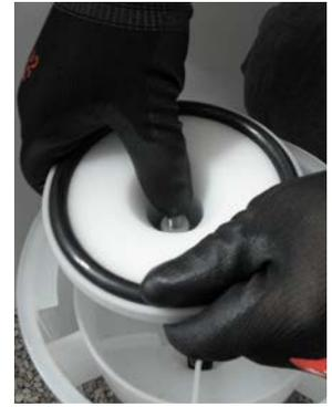
5.5 Clean and flush the slots of the basket on the valve disc.
