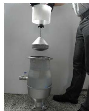
5.4 Unscrew the guide rod and press out the screw while simultaneously lifting the valve disc. Remove the valve disc.
