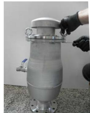
5.2 Lift the flange vertically upwards.
