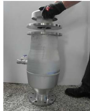
5.3 Pull the complete valve mechanism upwards out of the housing using the two handle straps and place it upright on a firm surface.
