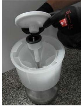
5.6 Pull out the diaphragm by tightening the stainless steel screw and check for sedimentary deposition and mechanical damage. Remove sedimentary deposition by wiping with a damp cloth. If it is necessary to replace the diaphragm, separate the diaphragm from the retaining groove and replace it with a new diaphragm. Also check upper sealing ring for sedimentary deposition and mechanical damage. If necessary, clean or replace with a damp cloth.
