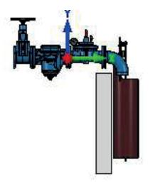
Hawido floating valve type 1600 can be used together with an opening limiter.
