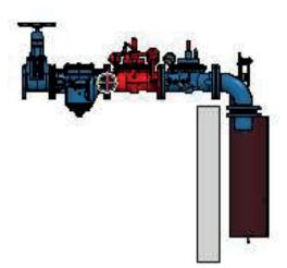
If the pressure is between 9 to 16 bar, a Hawido pressure reducing valve is required before the floating valve.
