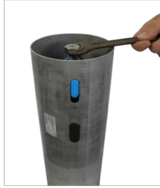
3. Loosen the centering screw.
