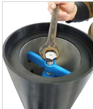
11. Screw down the centering screw until the air valve is filled with water.
