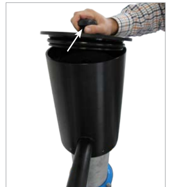
12. Put the lid onto device and fix it by means of the clamping screw.
