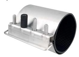
Pipe repair clamp with self-centring locking system for cast iron, steel, PVC and AC pipes. The screws welded to the clamping bridge allow easy assembly using the saddle strap. To facilitate installation, the central threaded pin is longer for d 87 mm and higher. The nuts can be screwed on easily from the supplied nut magazine, thus saving time.
