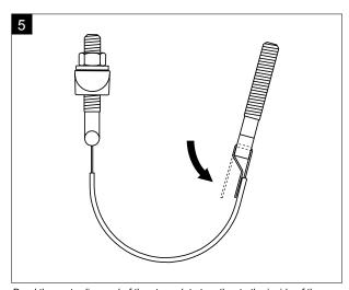
Bend the protruding end of the strap plate together to the inside of the plate.
