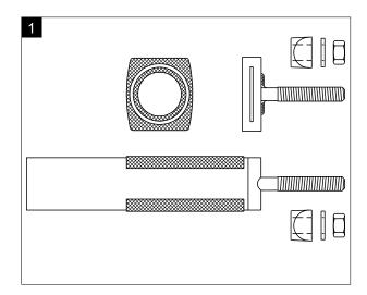
Check the completeness of the strap individual parts. Universal strap piece, clamping jaws, saddle seals, assembly T-piece, hexagonal nuts, clamping jaws, washers.
