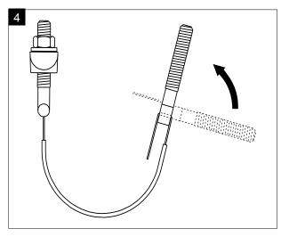
Bend the strap plate and assembly -T - piece further by 90° to the left.
