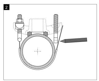
Mount the strap, hang it on the saddle body and bend it around the pipe. Position the assembly T-piece. Marking of the bending position on the sheet metal strip and the marking for cutting to length (bending position + min. 100 mm).
