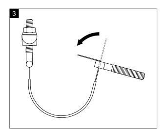
Fix strap and assembly T-piece together. At the marked position, bend the protruding strap plate end 90° to the pipe side along the assembly T-piece.
