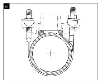
Hang the strap on one side of the saddle body and bend it around the pipe. Mount the second clamp. Tighten the hexagonal bolts with the specified torque (60 - 70 Nm / max. 100 Nm). Do not use an extension! Perform pressure testing.
