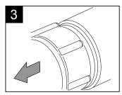
Apply approved lubricant Turn the ZAK® connection Pull back ZAK® connection as it will go.
