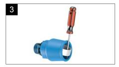
When reusing the fitting, replace the grip ring. Inspect O-ring seal and replace if necessary.
