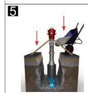
Before starting the filling work, please double-check the correct fit of the drainage element.
