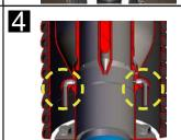
The hydrant is surrounded by a seeping water drain packing.
