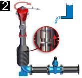
Close the hydrant after operation. Check the drain-off function. If the hydrant is not drained after a waiting period of four to five minutes, the clogged drain-off bore has to be flushed free, for example by means of a hand pump. Mount the cap for coupling A and/or B.
