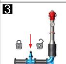
For maintenance work we recommend installing a gate valve into the branch line to the hydrant.
