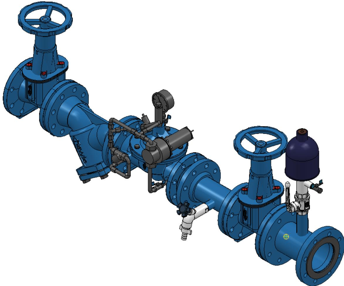
The HAWIDO must be installed horizontally with the valve cover upwards (other models available on request). We recommend that a gate valve and a dirt trap be fitted in front of the valve, as well as the mounting of an gate valve at the outlet.
