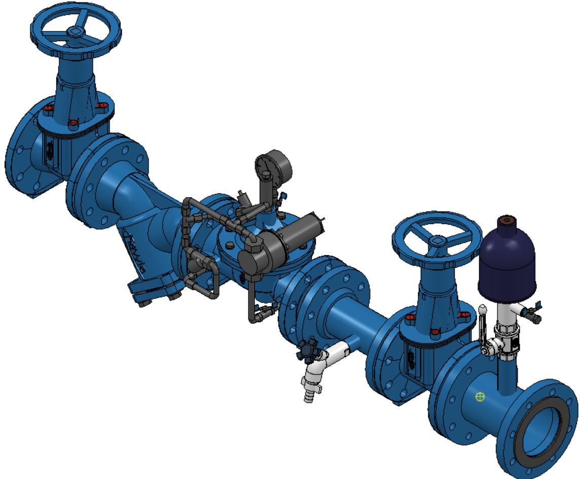
Regulating valves are normally fitted with the valve cover upwards. It is recommended that shut-off valves be fitted on both sides plus a dirt trap on the inlet side. Depending on the installation situation, a mounting adapter may also be required. If the HAWIDO 1400 is used as a relief valve, the shutoff gate valve on the outlet side can be omitted. Before commissioning, a check should be made that no coarse foreign bodies can penetrate into the HAWIDO.
