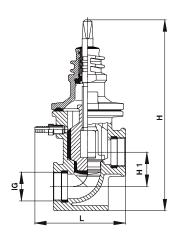
Resilient seated house connection drain valve with female thread on both sides to DIN ISO 228-1 and automatic drain.
