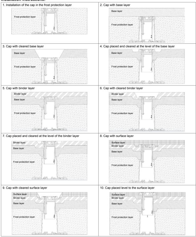
Note: Sectional drawings with surface box Order No. 187-01 shown!
