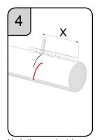
Mark the required insertion depth X on the pipe according to the table.
