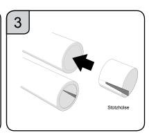
**IMPORTANT:** When PE pipes are connected, make sure to always use a Hawle support liner.
