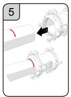
Push the pipe into the socket up to the max. insertion depth, but not as far as it will go.
