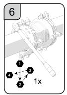
Bolts must not be lubricated. Tighten the bolts crosswise (see table) using a torque wrench.
