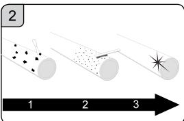
Before installation, clean the pipelines and remove dirt and foreign matter. The pipe surfaces must be smooth and clean, as well as free from grooves and corrosion.
