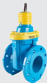
400-00G Flanged gate valve "E3", short, standard series 14 acc. to DIN EN 558-1
