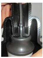
(Upper air valve part in cut sample view)
