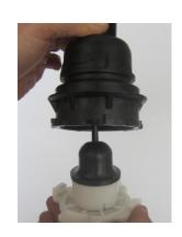
5.6 Roll diaphragm out and lock for remains of debris or mechanical damages. Remove debris with a wet towel. In case a change of the whole diaphragm is necessary, remove use diaphragm from the groove and replace it by an unused diaphragm.
