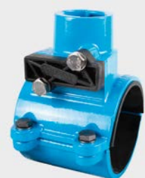
Clamp saddle with auxiliary shut-off facility: Shut-off effected by means of a shut-off blade of stainless steel, lateral drilling or drilling from above possible
