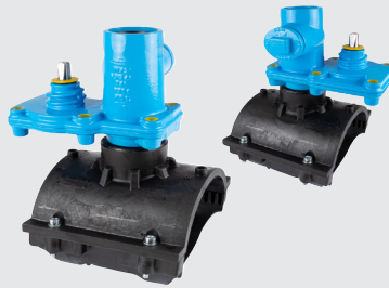
235-02G Weld-on Hawlinger with horizontal internal thread outlet, 90° angle to pipe direction
