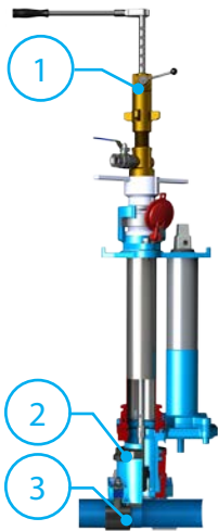
Drilling under pressure
