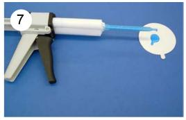
Then, upon discharge, the individual components are forcibly mixed homogeneously by the mixing elements in the mixing tube.
