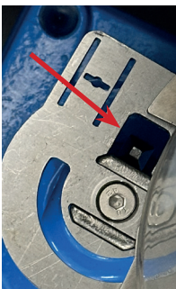
Image 3: Replacement valve assembly (6) locked:
