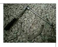
If a hydrant DN 80 with spigot end is installed in the socket, the socket must be turned to a 45° position. The hydrant is then inserted. To lock the socket, place the turning tool on the lateral bolts and turn the socket counter clockwise with the ratchet until the hydrant is locked. The anti-rotation device and dirt cap supplied must be fitted to prevent unintentional twisting and contamination.
