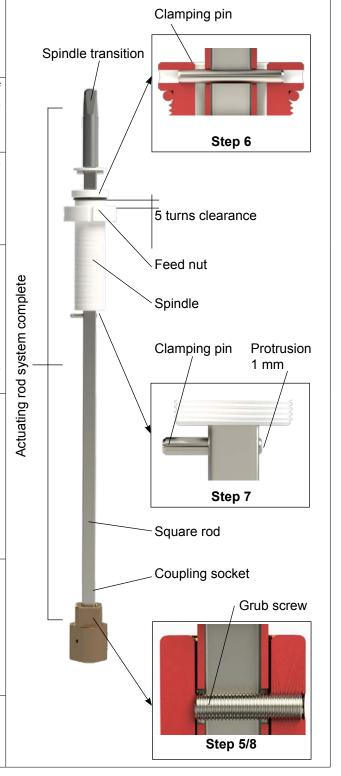
Mount the actuating rod in the standpipe; align the longitudinal groove of the feed nut with the guide rod of the standpipe, and push the actuating rod into the standpipe.
