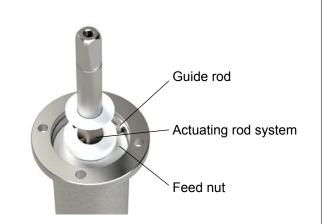
Mount the slide ring (tightening torque 0.5-1 Nm), position indicator "Auf / Open" and "Zu / Close" on the standpipe. To adjust the position indicator (Step 13), it is necessary that the position pointers can be moved on the pipe.
