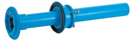
For the quick construction pipe entry connection with protection pipe, medium-conducting PE pipes (PVC on request) are pushed through the pipe entry connection into the inside of the building and connected with restraint via a push-fit fitting.
