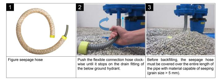
Seepage hose for Hawle freeflow underground hydrant set and Above ground hydrant H4 Ord. No. 514-00, 515-00, 517-00, 519-00 Ord. No. 490-10
