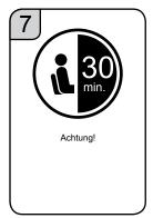
Retighten bolts after 30 minutes and/or after pressure testing
